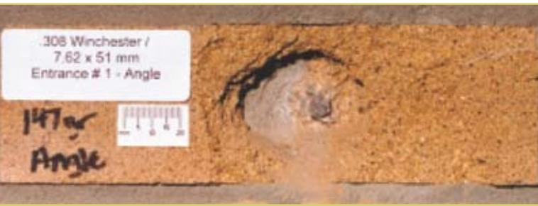
Above photo shows entrance point of impact. Bullet failed to pass through brick wall.
