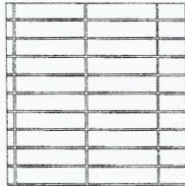
BLOC_NOBLE_400_100 _STACK-BOND Stacked Bond Pattern
